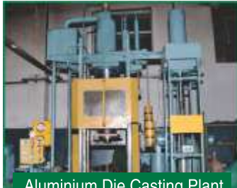
Aluminium Die Casting Plant
